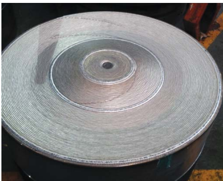
▲ Inconel cladding of crown top surface
