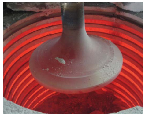
▲ Heat treatment of valve spindle
