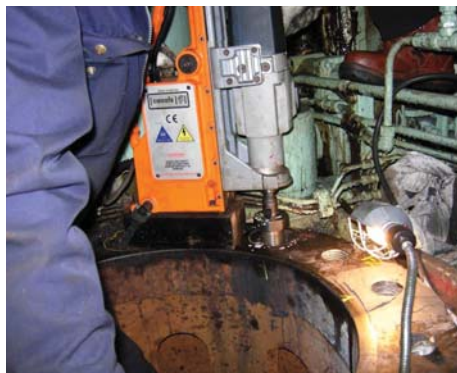
▲ Cyl. Cover Stud. Modification
