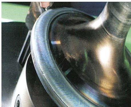
▲ Valve spindle - disc seat welding
