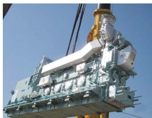
Aux. Engine Replacement ▶
