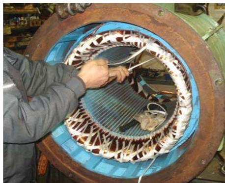
▲ Rewinding of bow thruster motor
