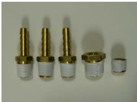
FIGURE 2. APPLY THREAD SEALANT
